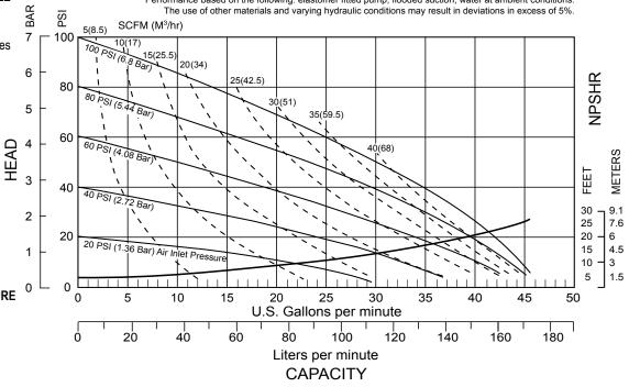
Performance based on the following: elastomer fitted pump, flooded suction, water at ambient conditions.
