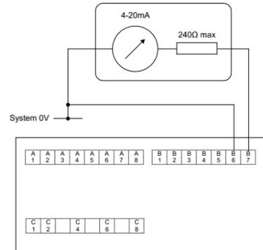
Note: Modbus, USB and Analogue 0V lines are internally connected.
