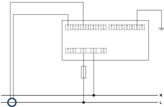
Ensure CT is fitted correctly for direction of energy flow – labelled side should face the power source and non-labelled side faces the motor.
