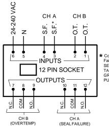
\* Connection for 2 Wire Seal Fail Shown. ON 1 WIRE SEAL FAIL CIRCUITS, ATTACH PIN 3 TO COMMON GROUND POINT WITH PUMP GROUND WIRE.
