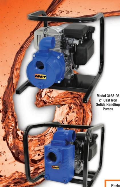
The AMT line of Engine Driven Solids Handling pumps offers an upgraded debris handling capability in wear resistant cast iron construction. Applications include: high volume liquid transfer, irrigation, commercial draining and construction. All models feature durable all cast iron construction and clog-resistant impeller to ensure a long life for the complete pump. Dual volute design reduces radial load on engines.
